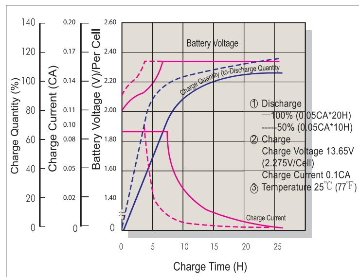
**Terminal Voltage (V) and Discharge Time (25°C 77°F)**
