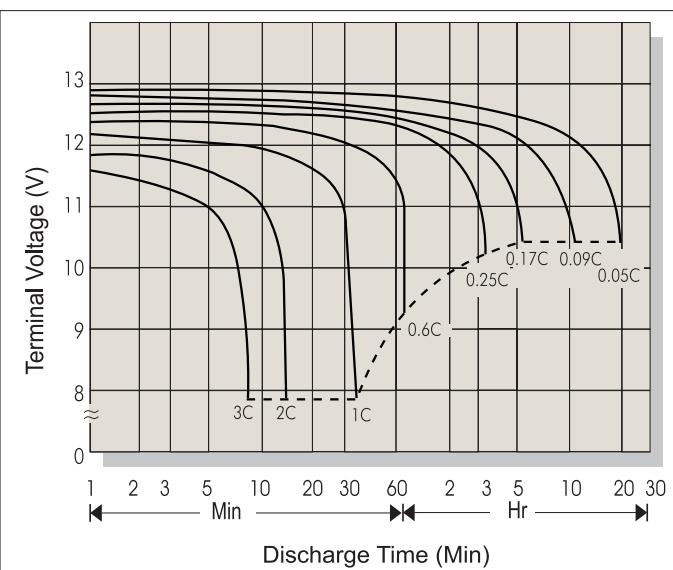
**Battery Voltage and Charge Time for Cycle Use**
